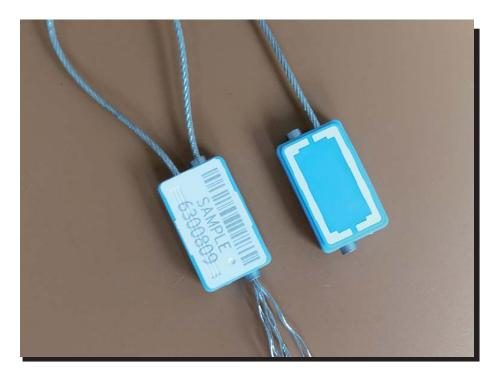
In the production process, the white part is not welded, it is directly injection, and the white plastic goes through from the front side to the other side to wrap the whole lock housing, so the white part is impossible to be pried open.
